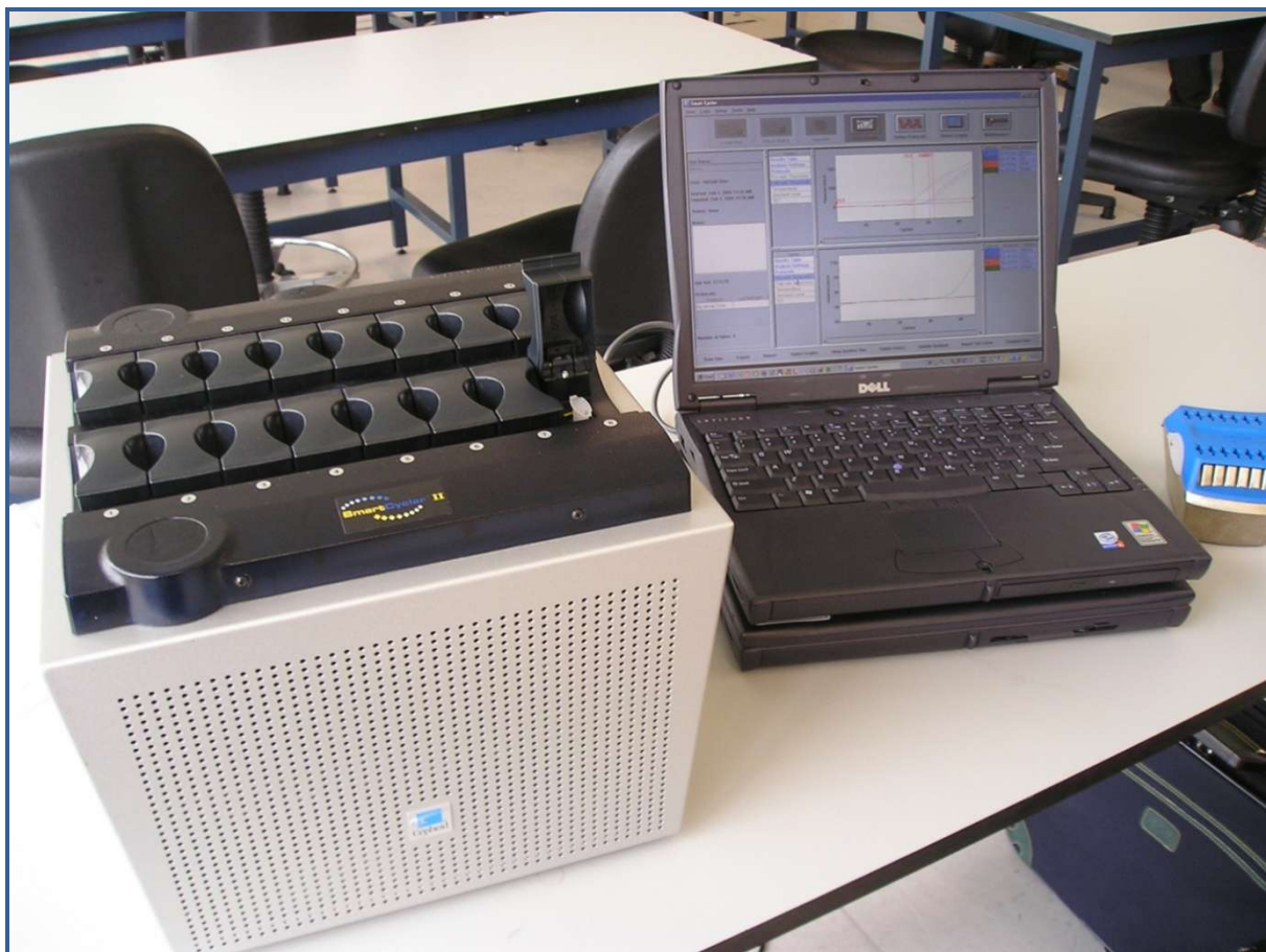
Fig. 4.1.1.4: SmartCycler (Cepheid), a portable thermocycler allowing the use of real time PCR in the field, at ports, other entry points and other points of interest. Using a modified real time PCR Ams assay, results can be obtained in less than 40 minutes with sensitivity comparable to laboratory conditions.
