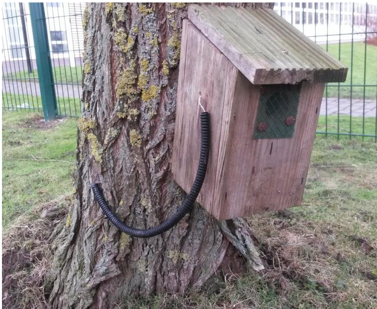
Fig. 2.5: Bird box used to house the temperature logger and lead going into the tree trunk surrounded by plastic as rodent protection
