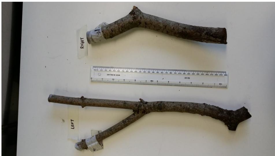
Fig. 2.2: Wood samples set-up for simultaneous audio recordings of ALB larval feeding
